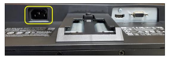
3. Connect the female end (circled below) of the power cable to the monitor.
