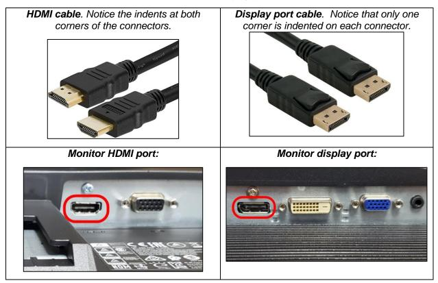
2. Connect the other end to either HDMI or display port on the back of the PC.
