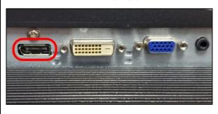
2. Connect the other end to either HDMI or display port on the back of the PC.
